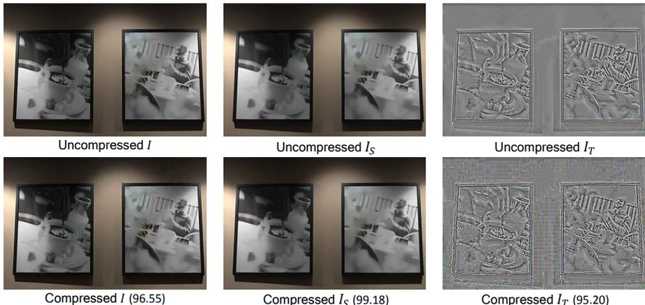
**Fig. 3.** This shows two examples of structure-texture decomposition in uncompressed and compressed image ( $Q40$ ) pairs. The structure similarity index measurement (SSIM) [24] values (in  $\times 100$  scale in the paper) between each pair are shown in the brackets. Notice that most of the characteristic compression artifacts exist in the texture layer, while the structure layer of the compressed image resembles that of the uncompressed image.
