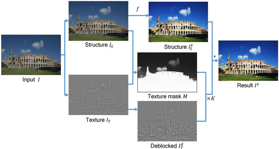
**Fig. 2.** The overview of our proposed method. The input image is decomposed into structure and texture components. The contrast of the structure component is then boosted directly; the texture component that contains the JPEG artifacts is processed to reduce compression artifact. The two components are recombined at the last step to render the final result. In the paper, we amplified the textural part by a factor of 10 and shift it by +0.5 for better visualization.
