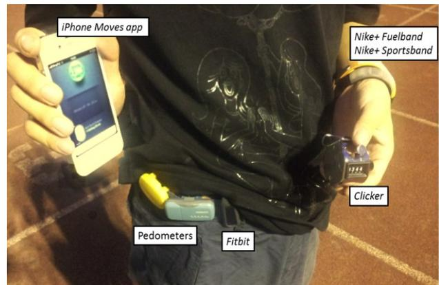
Figure 2. A participant in our study wearing multiple devices. A mechanical clicker was used to record number of steps.
