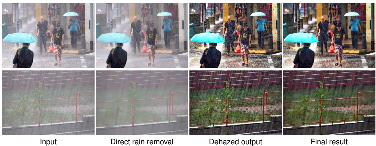
Figure 6: Rain streak removal example for heavy rain. We found that first applying a dehazing method (3rd column), followed by the rain streak removal, helps improve results.
